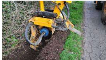
Tractor Mounted Grip Cutting Head
